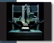
Scorpion Robot Inspection is an area where Scorpion excels using a robot to move 2D or 3D cameras to capture multiple high resolution and high quality images of parts.
